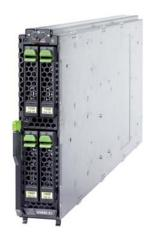
integrated, highly functional SAS/RAID controllers with optional 512 Mbyte cache and BBU. Each controller provides RAID levels 0, 1, 5 and 6. The connection to each Server Blade is realized via a midplane link to the high performing PCIe x4 interfaces of each Server Blade's system board.
